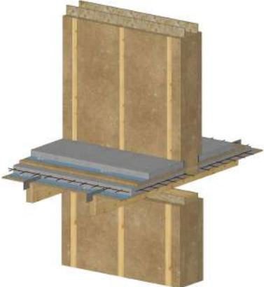
A 3D cutaway diagram showing the installation of a floor slab (grey) with acoustic insulation (yellow) between the slab and the wall. The wall is made of a light-colored, textured material. The slab is supported by a blue metal bracket or reinforcement. | Einbau der Trittschalldämmung   |
